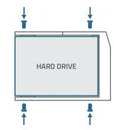
3. Fix your hard drive to the bracket with the provided screws.
