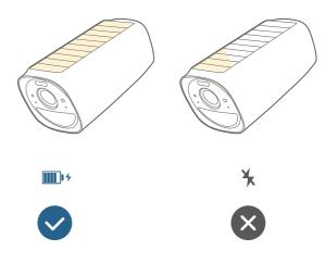
\* Make sure the solar panel can be fully exposed to direct sunlight for at least 2 hours per day.
